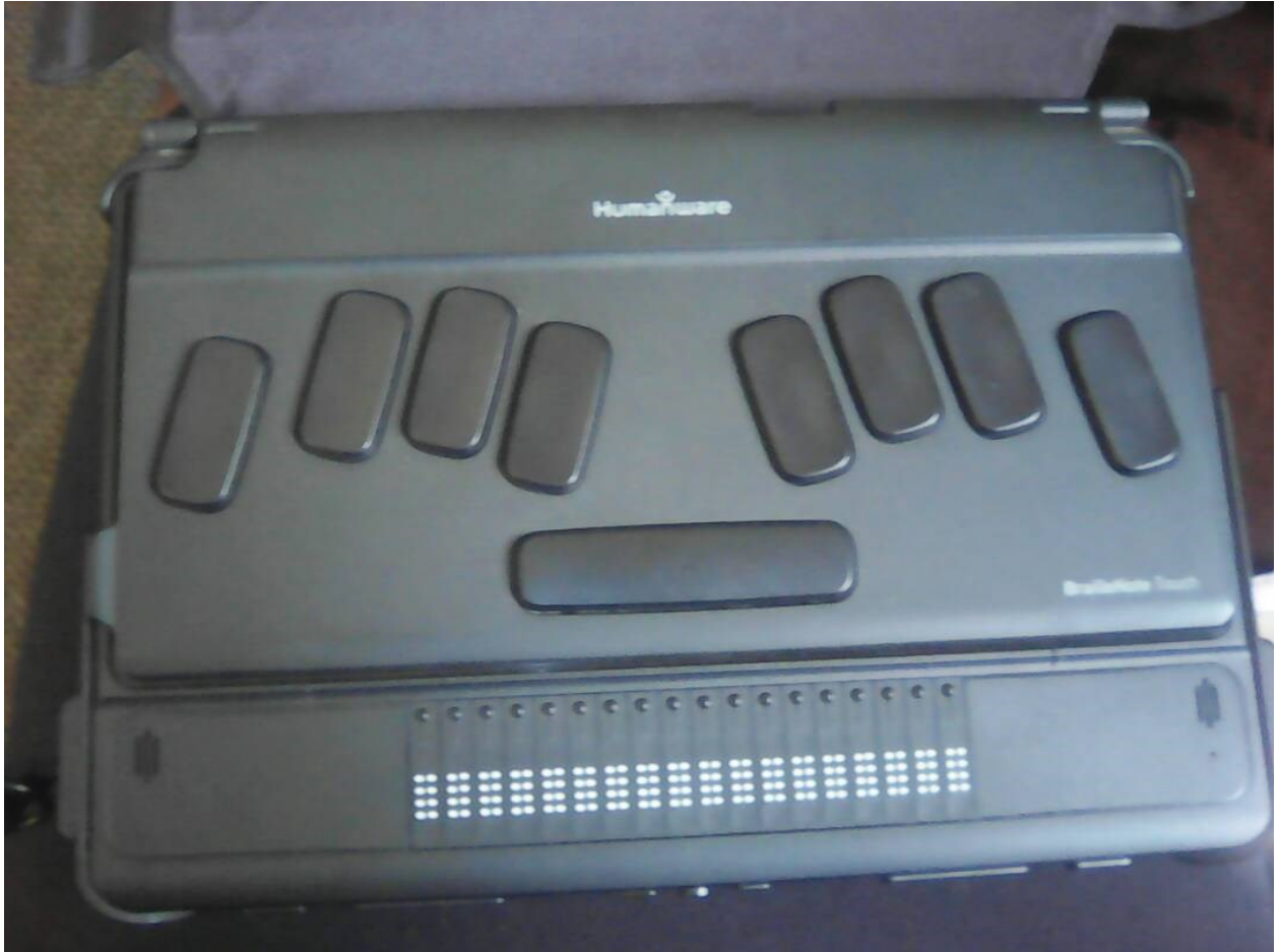
Figure 13 Photograph of a Braille Note Touch Note Taker for the visually impaired. The user can use it to type on a Braille keyboard or to read, so it can be used interchangeably. It can also be used as a keyboard if it is connected to a computer. It enables fast and convenient typing.
