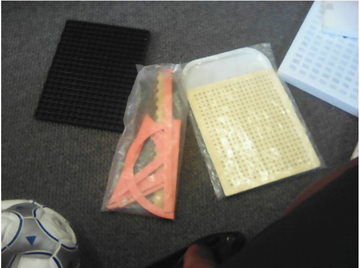
Figure 14: Photograph of a writing board used by the visually impaired to write notes in Braille. It comes with a Braille alphabet.
