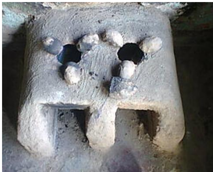
Figure 5: Photograph of an energy saving stove being promoted by one of the organisations working in Ndirande, Blantyre Urban
